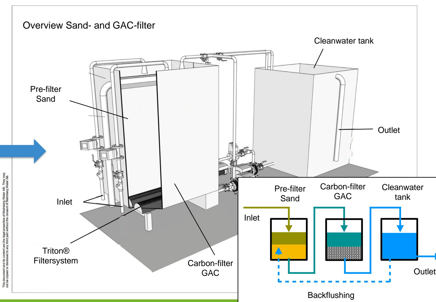
The same type of filter as the one described to the left will be connect to the WWTP effluent. The GAC-filter will be placed right after the already existing sand filter at Degeberga WWTP. The estimated costs are shown below.
